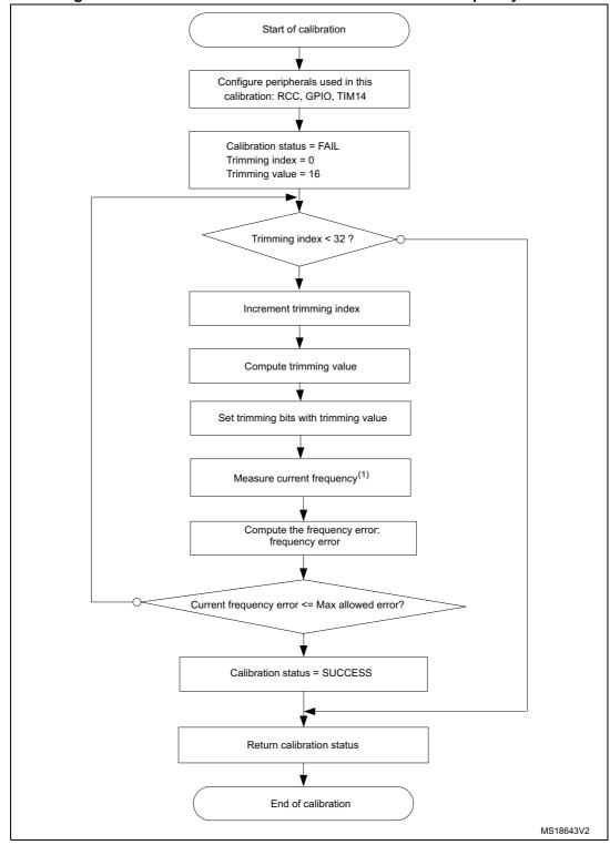
Figure 12. HSI calibration flowchart: maximum allowed frequency error
