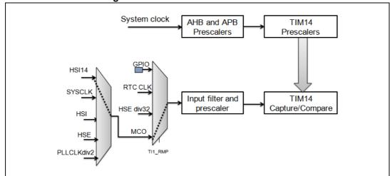
Figure 9. Hardware connection For HSI14
