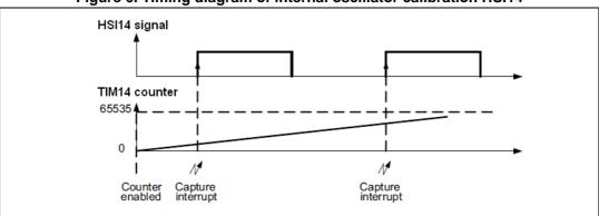
Figure 6. Timing diagram of internal oscillator calibration HSI14
