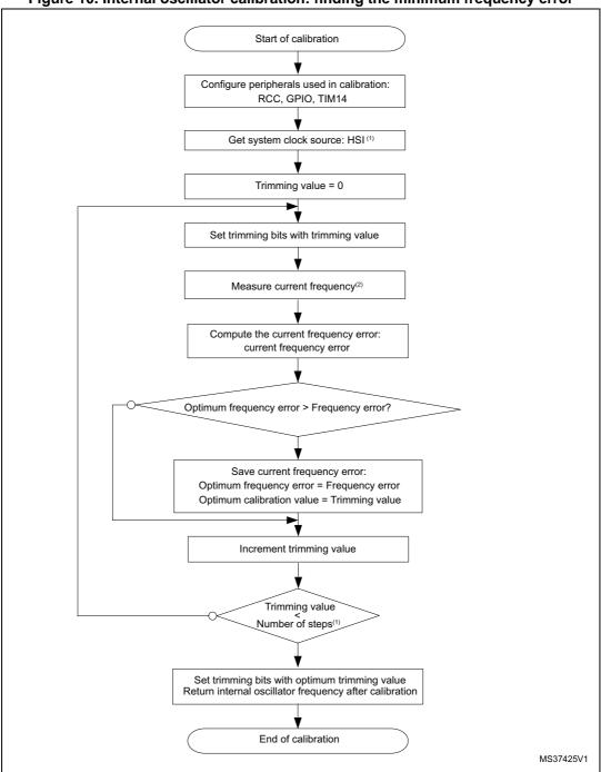
Figure 10. Internal oscillator calibration: finding the minimum frequency error
