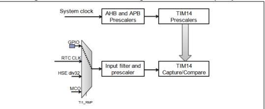
Figure 8. Hardware connection using external reference frequency
