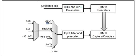
Figure 14. LSI measurement configuration
