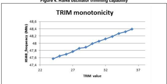
Figure 4. HSI48 oscillator trimming capability
