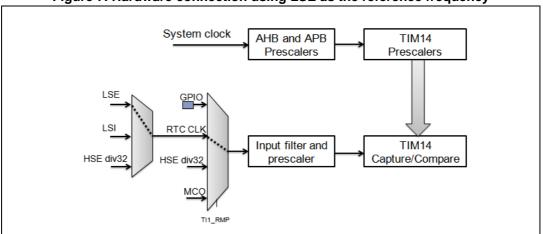
Figure 7. Hardware connection using LSE as the reference frequency
